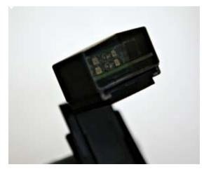
The T-eye Drive Recorder is an in-car video recorder that captures footage both inside and out. It has two CMOS VGA (640x480) cameras that each offer 170 degree viewing angle (making for a total 340 degrees). Video is recorded in Motion JPEG at 16 frames per second. With the supplied 2GB SD card it can record up to 60 minutes, or 90 minutes at lower resolution. The unit can also support 8GB and 16GB cards, which equates to 12 hours of footage on the 16GB.
