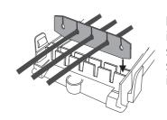
Next, place the rubber seals with the now inserted cables into the slot, as depicted in the example on the left. Make sure the rubbers are pushed down all the way using silicone spray to facilitate this. Put the lid back on so that it is tight and secure.
